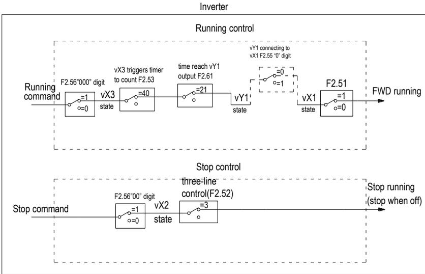
**Notes:** It can be seen from the above figure that the actual method requires access to two actual external X terminals. If virtual terminals are used, no external actual terminals need to be connected
