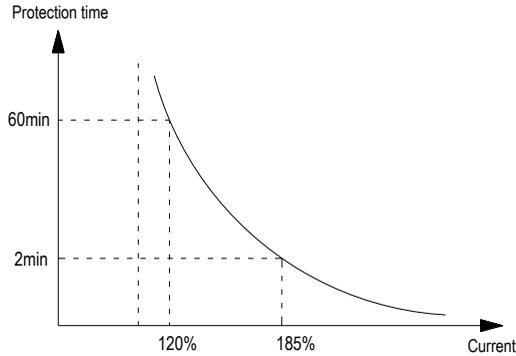
The current entering protection curve= (the real motor current / oL protection coefficient)x110%
