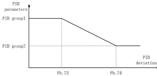
Switching the PID parameters according to the deviation
