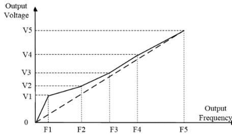
User sets the 1<sup>st</sup>/2<sup>nd</sup>/3<sup>rd</sup>/4<sup>th</sup>/5<sup>th</sup> voltage ratio of V/F curve corresponding to F1/F2/F3/F4/F5 frequency based on rated output voltage 100%. User sets the 1<sup>st</sup>/2<sup>nd</sup>/3<sup>rd</sup>/4<sup>th</sup>/5<sup>th</sup> frequency of V/F curve corresponding to V1/V2/V3/V4/V5. Must meet:  $0 \leq F1 \leq F2 \leq F3 \leq F4 \leq F5 \leq \text{max frequency}$ ,  $0 \leq V1 \leq V2 \leq V3 \leq V4 \leq V5 \leq 100.0\%$
